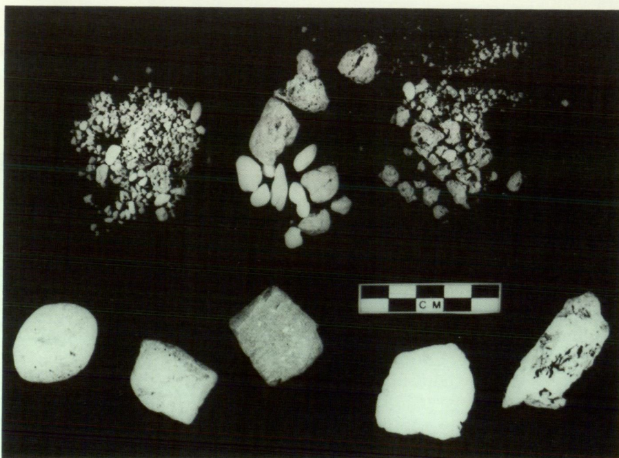
Figure 5 Clasts from the fossil bone bed, Lancefield swamp. The sediments are highly unsorted, atypical of swamp deposits. Scale in centimetres.
